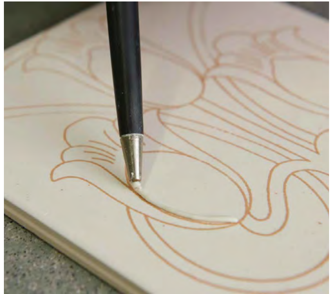
2. The pattern is stenciled onto the blank tile biscuit (this one is Liberty). A thin line of slip is carefully piped following the stencil lines – just like icing a cake
