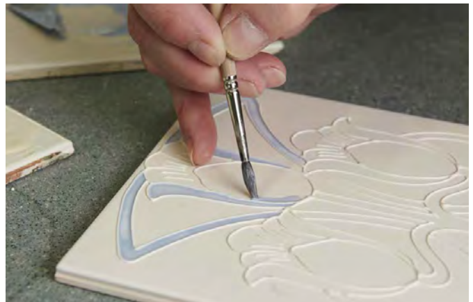
3. When the piped outline has dried, coloured glazes are hand painted in separate areas within the lines. As you can see, the glaze colour does not resemble the finished tile
