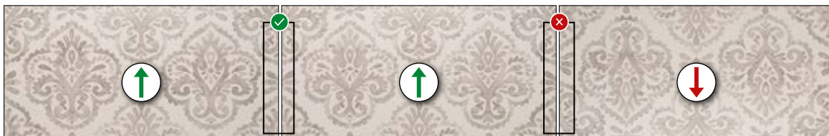
example of correct and incorrect alignment
